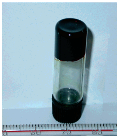
Figure 6. Photograph of the SNC electrolyte (0.18 M I 2 , 1.3 M BMI·I, 0.5 M LiI, 1 M 4- tert -butylpyridine in BMI·BF 4 , 5 wt % silica nanoparticles) at 85 °C.
